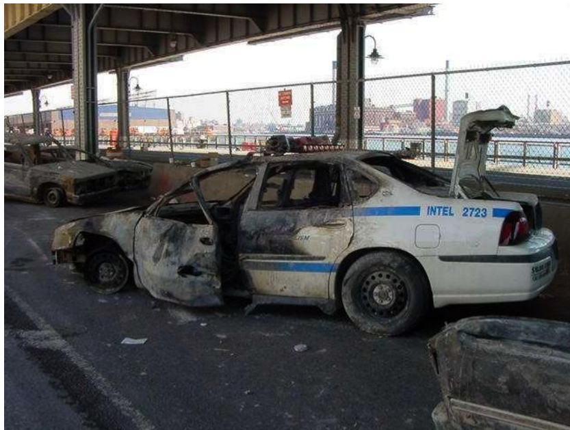
Figure 40. There is extensive damage to the front of car 2723, including no door handle on the driver's door. There is an unusual, unburned circular area on the rear door.
