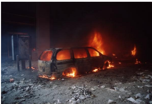
Figure 50. A mini van is consumed by flames. The fire rages inside the vehicle, contained by the remaining windows. The fire appears more intense at the front where the engine is.
