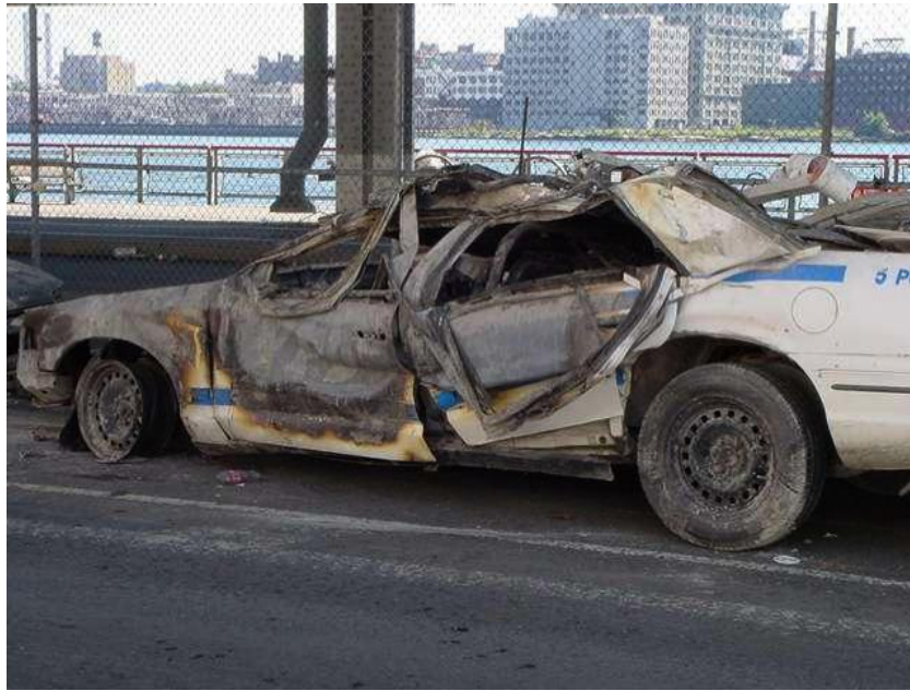
Figure 39. Peculiar wilting of car doors and deformed window surrounds on FDR Drive.
